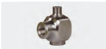
3/8" IG : 3/8" AG. DN 10. Max. 30 U/min / 90 °C
