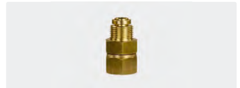
3/8" AG : 1/4" IG. Messing. Max. 220 bar / 90 °C
