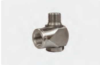
3/8" IG : 3/8" AG. DN 6. Max. 400 bar / 30 U/min / 90 °C
